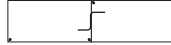
End to end, opposite facing: 36"d & 30"d, use 28" jumper. 24"d & 18"d, use 24" jumper.
